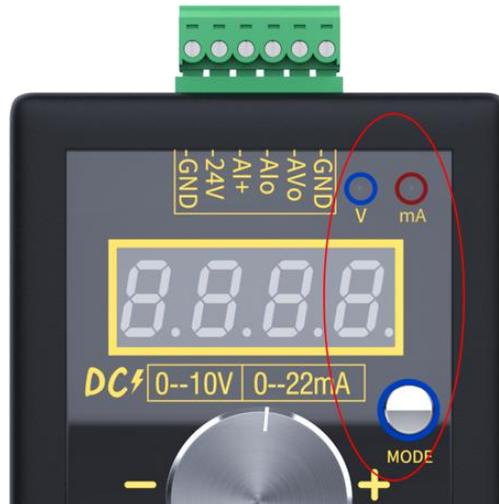
Press the MODE button, one key switch to adjust the voltage and current mode; The indicator shows what state it is in, System operation corresponds to which mode to operate; The original mode after switching, Will continue to output, It's just not in a state of adjustment;
